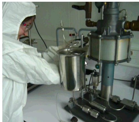
Fig. 3. C. de Gracia-Lux operating a high-pressure microfluidizer for fluorocarbon emulsion preparation.
